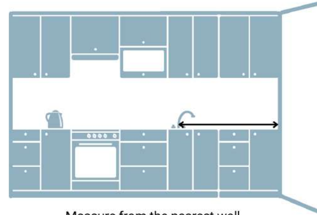
3 Measure from the nearest wall to the center of the sink faucet.
